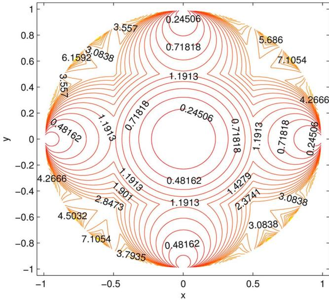
Fig. 6. Gap  $\gamma_{I,H}$  (in dB) for the complex two-tap channel  $H(D) = 1 + (x + j \cdot y)D^p$ , when the optimal integer-valued filter  $I(D)$  of length smaller than (or equal to)  $5(p + 1)$  is used.
