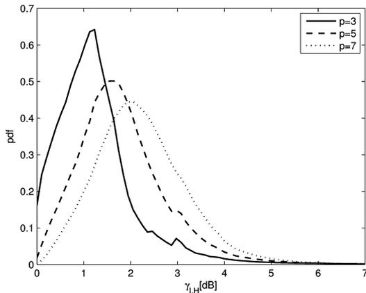
Fig. 7. Probability density function (pdf) of  $\gamma_{I,H}$  (in dB) for the ISI channel  $H(D) = \sum_{k=0}^p h_k D^k$  where  $\{h_k\}_{k=0}^p$  are i.i.d. random Gaussian variables with zero mean and unit variance, when the optimal integer-valued filter  $I(D)$  of length smaller than (or equal to)  $5(p + 1)$  is used.
