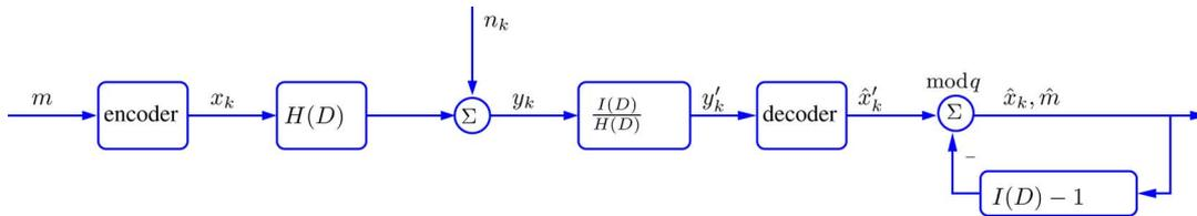
Fig. 2. High-level schematic description of an IF-DFE system (assuming  $i_0 = 1$ ).
