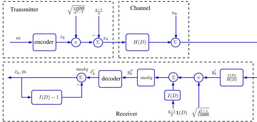
Fig. 4. Detailed description of an IF-DFE system (assuming  $i_0 = 1$ ).
