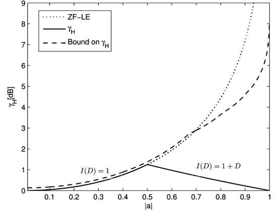
Fig. 5. Gap  $\gamma_H$  for the real two-tap channel  $H(D) = 1 + aD^p$ . The solid line shows  $\gamma_H$  for any value of  $p$ , the dashed line shows the bound (30) for  $p = 1$ , and the dotted line shows the noise enhancement induced by ZF-LE.
