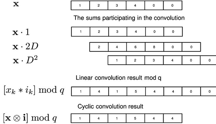
Fig. 3. Illustration of the equivalence between a linear convolution  $x_k * i_k$  and a cyclic convolution  $[\mathbf{x} \otimes \mathbf{i}] \bmod q$  when the last  $n - 1$  entries of  $\mathbf{x}$  are zero. In this example,  $I(D) = 1 + 2D + D^2$  and  $q = 7$ .
